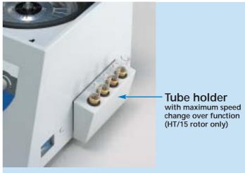
In case where the centrifuge is used for the hematocrit, 15mL metal tubes should be inserted into the tube holder attached to the side cover of the centrifuge as shown in the photo. In case where 15mL glass tube is used, take the 15mL metal tubes out of the tube holder and mount on to the rotor. If so, the speed is limited to 4,000rpm.
