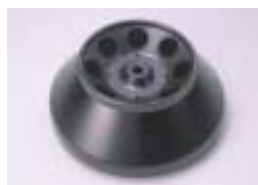
RA-410M3 8 x 50/15mL Conical tube This rotor is not a tool-less rotor.
