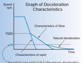
The switch over point of N to the natural deceleration can be selected from 0 to 15,000 rpm.
